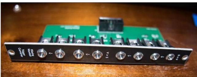
Turn the PCB and solder the audio jacks onto it.
